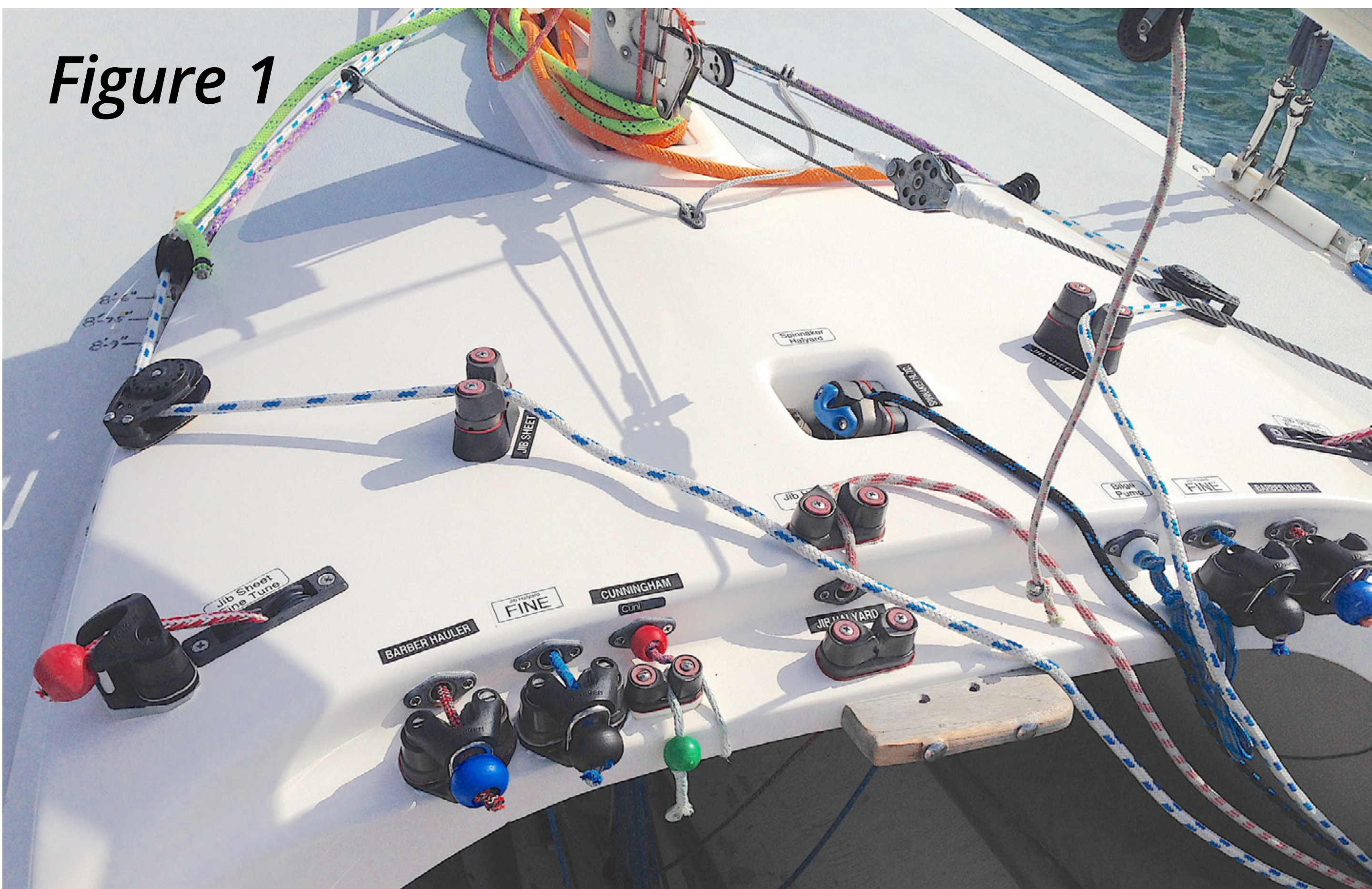
Figure 1. Control lines on cuddy; note jib sheet barber hauler pulls on fine-trim part of sheet tackle.
